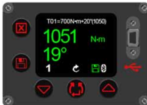
FIGURE 53 – Torque & Angle target (with Final Torque) result (shown as green for pass)
