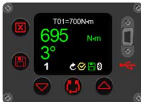
FIGURE 54 – Audit Torque target result (showing achieved torque and output (bolt) movement in degrees)
